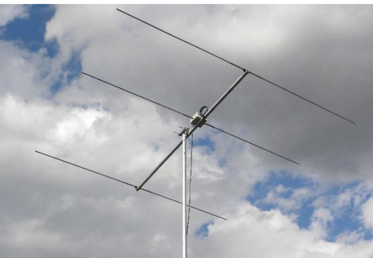
3 Element 70 MHz Yagi Antenne
